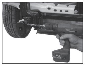
8. If no drilling is needed proceed to step 10, On models where drilling is needed, drill 1/2" holes on inside of frame using holes as template. Slide baseplate between frame horns(If there is a gap between frame horns and baseplate insert shim as shown on front page). Use the shorter metric bolts shown on front page (12mm-1.75 x 40mm Gr. 8.8). Top bolt on each side will go inward and bottom bolt will go outward as shown on front page.
